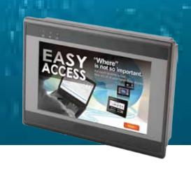
The PV-3070A utilizes an embedded 600 MHz microprocessor to provide crisp performance and startling HMI graphics. An aesthetically designed rigid aluminum enclosure offers anti-corrosion and effectively dust and dirt free protection.
