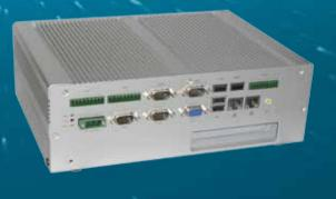
The SMART-T2100 Industrial Embedded Fan-less PC with Intel Atom D525 1.8GHz Processor
