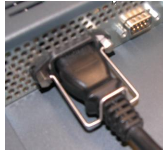
Power Cable Retention Clip Installed
