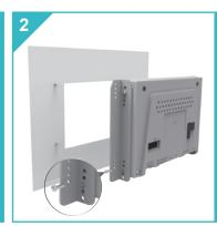
Select the mounting holes according to the wall thickness of control cabinet and secure the mounting brackets onto both sides of the HMI unit.
