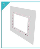
Around the cutout on the control cabinet, draw the reference lines for positioning the overlay.
