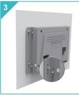
Secure the HMI to the cabinet by four studs.
