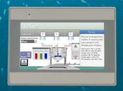
The PV-8050iE utilizes an embedded 600 MHz microprocessor to provide crisp performance and startling HMI graphics. An aesthetically designed plastic enclosure offers anti-corrosion and effectively dust and dirt free protection.
