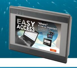
The PV-3070A utilizes an embedded 1GHz Cortex-A8 microprocessor to provide stunning performance and startling HMI graphics. An aesthetically designed rigid aluminum enclosure offers anti-corrosion and effectively dust and dirt free protection.
